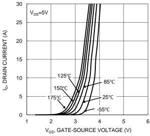
Figure 2. Typical Transfer Characteristic
