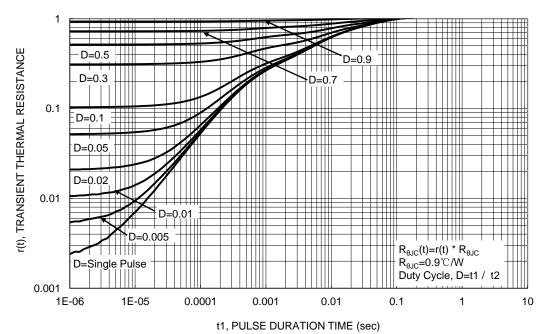
Figure 14. Transient Thermal Resistance
