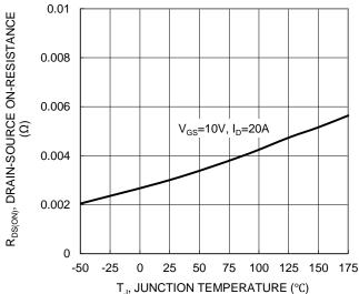
Figure 7. On-Resistance Variation with Junction Temperature
