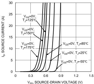
Figure 9. Diode Forward Voltage vs. Current
