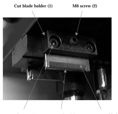
Fixed screw (3) Wire pusher (5) Wire cut blade (4)
