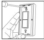
NOTE: For proper assembly, make sure to align the "top" labels on the rocker pad and wall plate.
