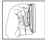
TIP: To remove the trim plate, use a flat-head screwdriver to depress the trim plate tabs using the 2 slots on the bottom of the wall plate. Alternatively, use a fingernail to press down along the top groove and flex the tabs out of the slots.
