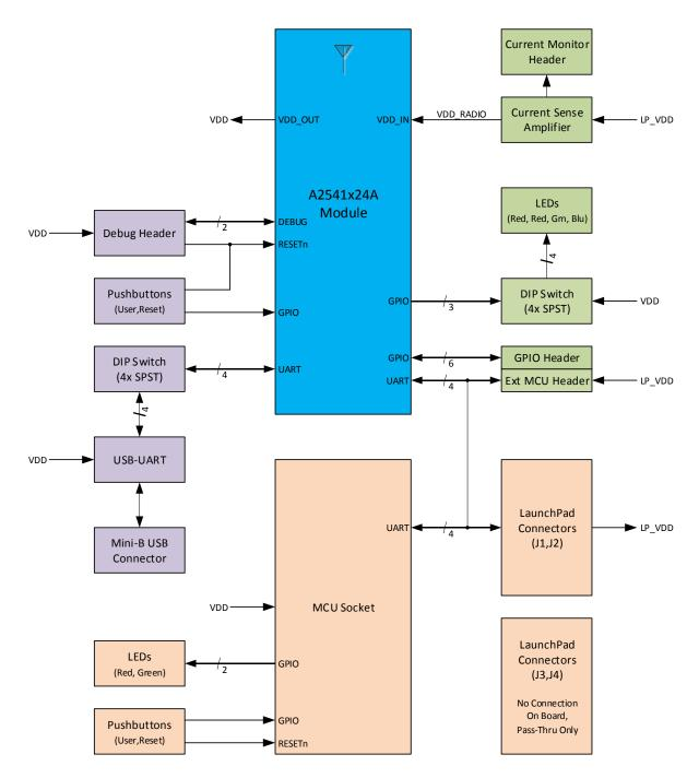
Figure 7 – Hardware Block Diagram
