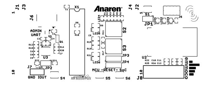
Figure 14 - PCB Layout Top Silkscreen
