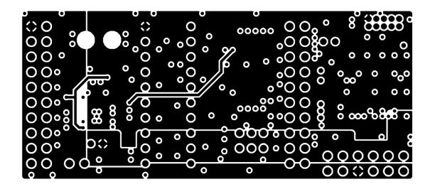
Figure 12 - PCB Layout Inner Layer (Split PWR Plane)
