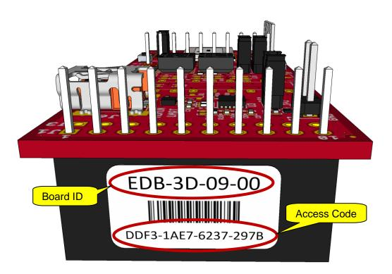
Figure 6 – AIR B-Smart BoosterPack ID Label
