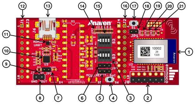
Figure 2 – AIR B-Smart BoosterPack Overview
