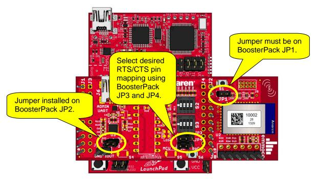
Figure 4 – AIR B-Smart BoosterPack Installed On MSP-EXP430G2 LaunchPad
