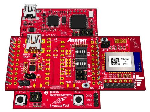
Figure 1 - AIR B-Smart BoosterPack with MSP-EXP430G2 LaunchPad
