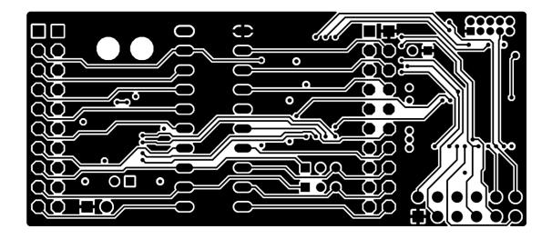
Figure 13 - PCB Layout Bottom Layer
