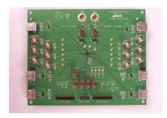
FIGURE 1. ISL540230EVAL2Z, ISL540230EVAL3Z EVALUATION BOARD
