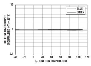
Figure 8. Relative Light Output vs Junction Temperature
