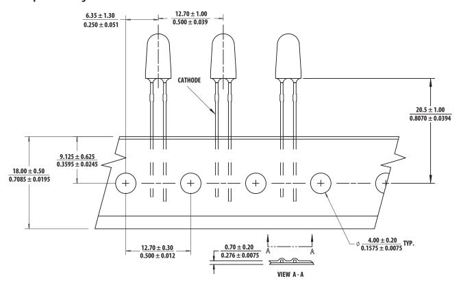
$Note: The\ ammo-packs\ drawing\ is\ applicable\ for\ packaging\ option\ -DD\ \&\ -ZZ\ and\ regardless\ standoff\ or\ non-standoff\ or\ no$
