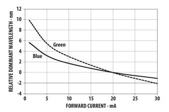
Figure 5. Relative dominant wavelength vs Forward Current
