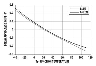
Figure 9. Forward Voltage Shift vs Junction Temperature
