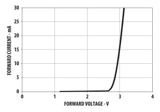
Figure 2. Forward Current vs Forward Voltage
