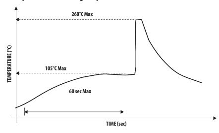
Recommended solder: Sn63 (Leaded solder alloy) SAC305 (Lead free solder alloy)
