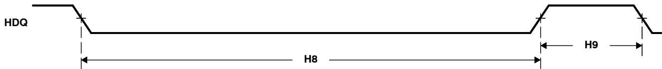
Figure 5-39. HDQ/1-Wire Break (Reset) Timing
