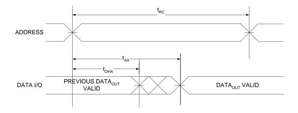
Figure 14. Read Cycle No. 2 of CY7C1061GE (Address Transition Controlled) [26, 27]
