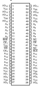
Figure 10. 54-pin TSOP II (22.4  $\times$  11.84  $\times$  1.0 mm) Dual Chip Enable with ERR CY7C1061GE $^{[6,\ 7]}$  Package/Grade ID: ZSXI
