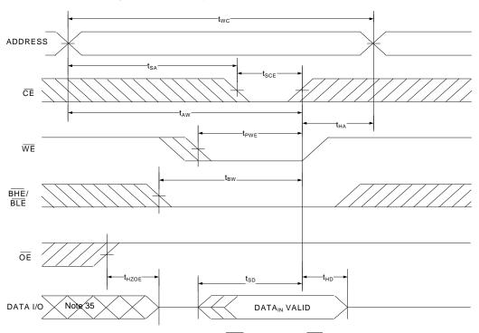
Figure 17. Write Cycle No. 2 (WE Controlled,  $\overline{\text{OE}}$  LOW) [31, 32, 33, 34]
