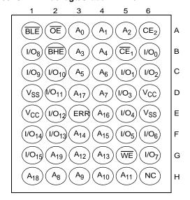
Figure 6. 48-ball VFBGA (6 × 8 × 1.0 mm) Dual Chip Enable with ERR, Address MSB A19 at Ball H6 CY7C1061GE<sup>[4, 5]</sup> Package/Grade ID: BVXI
