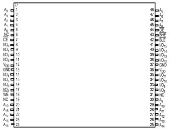
Figure 9. 54-pin TSOP II (22.4 × 11.84 × 1.0 mm) Dual Chip Enable without ERR CY7C1061G<sup>[6]</sup> Package/Grade ID: ZSXI
