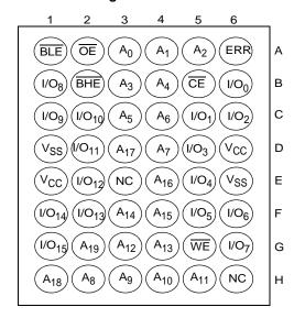
Figure 5. 48-ball VFBGA (6 × 8 × 1.0 mm)
