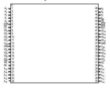
Figure 8. 48-pin TSOP I (12  $\times$  18.4  $\times$  1 mm) Single Chip Enable without ERR CY7C1061G<sup>[6]</sup> Package/Grade ID: ZXI
