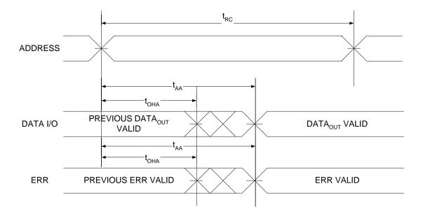
**Notes** 26. The device is continuously selected,  $\overline{OE} = V_{IL}$ ,  $\overline{CE} = V_{IL}$ ,  $\overline{BHE}$  or  $\overline{BLE}$  or both =  $V_{IL}$ . 27. WE is HIGH for read cycle.
