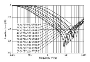
Common Mode Insertion Loss-Frequency Characteristics
