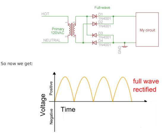
As you can see, there are twice as many humps - there isnt that "half the time, no voltage" thing going on. This means we can divide the calculated capacitor size to half of what it was in the previous.
