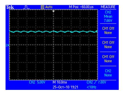
With 35 ohms (230 mA draw) the voltage plummets to 7.7V!
