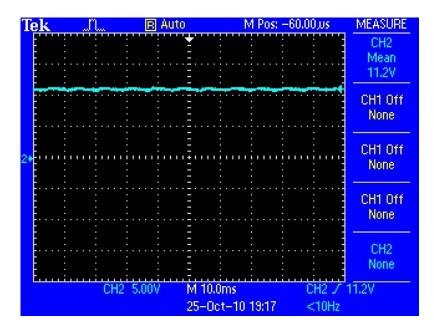
When I connected a 100 ohm resistor (110 mA draw) from the positive pin to the negative pin, it dropped to 11.2V
