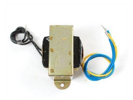
We aren't going to get into the heavy detail of the electromagnetic theory behind transformers except to say that they are made of two coils of wire around a chunk of iron. If the number of coils are the same on both sides then the AC voltage is the same on both sides. If one side has twice the coils, it has twice the voltage. They can be used 'backwards' or 'forwards'! For more detailed information, be sure to check out the wikipedia page (http://adafru.it/alf).
