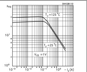
Figure 4. DC current gain NPN ( $V_{CE} = 1 \text{ V}$ ) Figu
