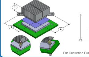
1) Dimension A is the length of the heat sink in the direction of the flow.
